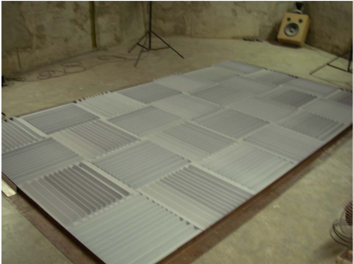
Figure 2: SoundAcoustics BA600-60 Foam Panels: Test Set-up. Note 90 degree rotation between adjacent panels.
