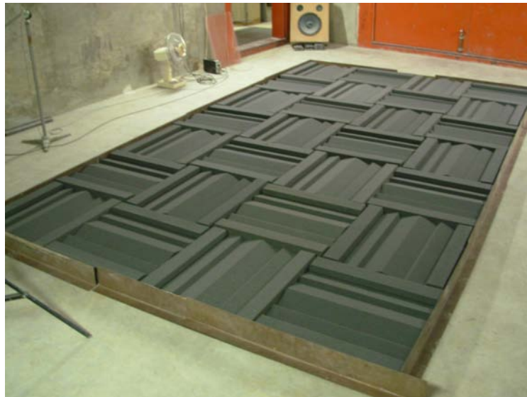
Figure 3: Sound Acoustics Hybrid Acoustic Panels with acrylic diffuser removed in the reverberation chamber.
