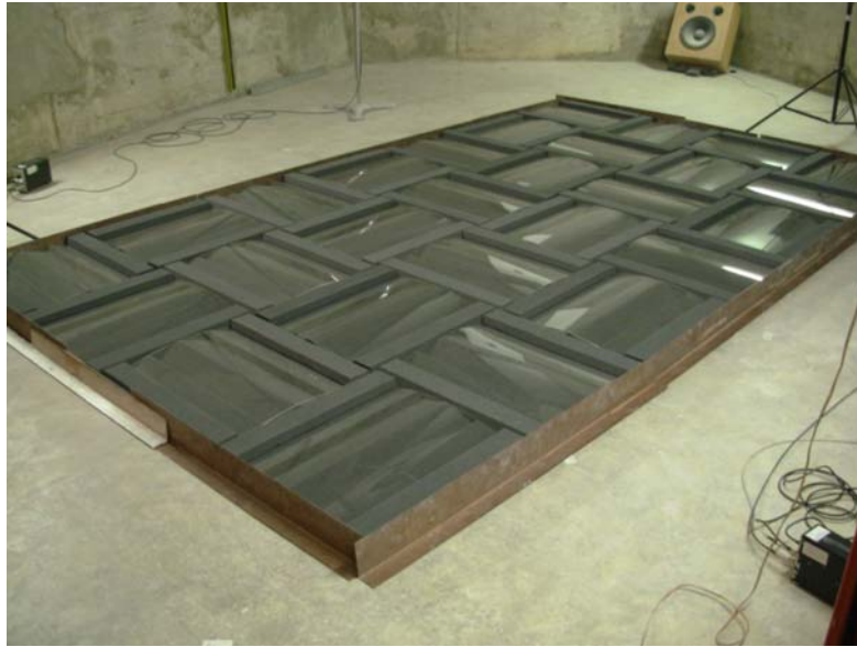
Figure 3: Sound Acoustics Hybrid Acoustic Panels with acrylic diffuser installed in the reverberation chamber.
